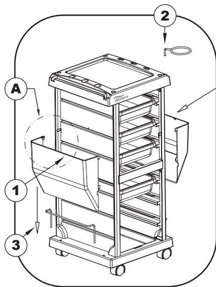
This trolley requires minimal assembly. Only the two side pockets, hairdryer holder and lower racks need to be attached.
